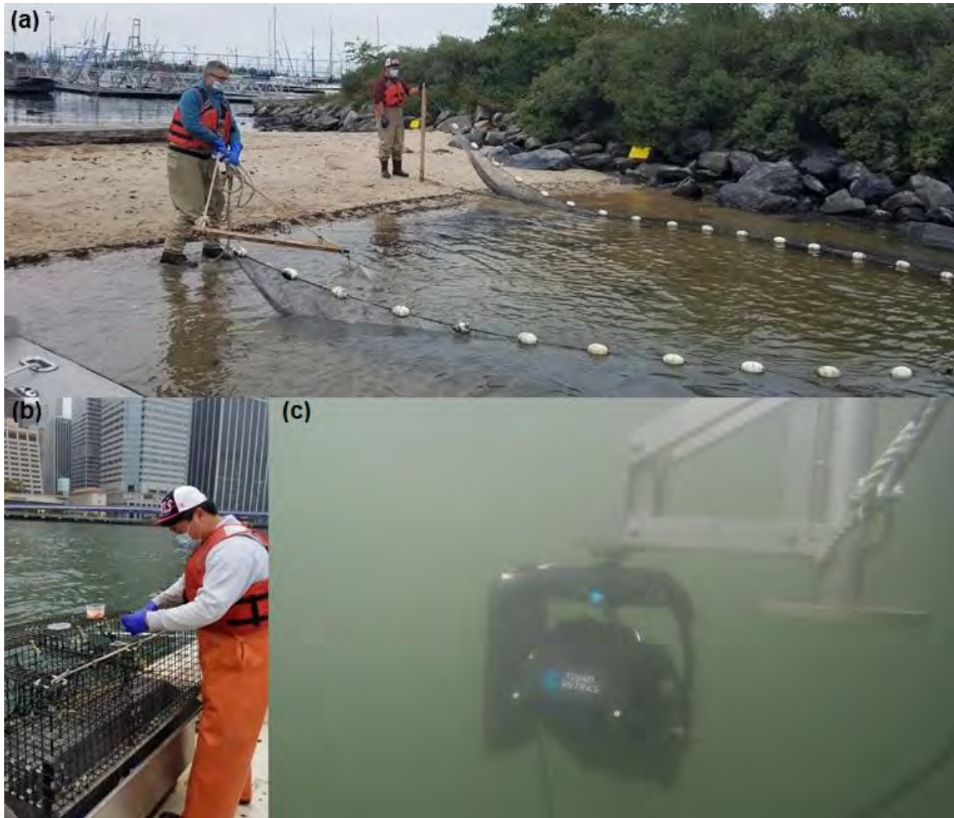
Figure 8 – Fish sampling by (a) beach seine, (b) baited trap, and (c) remote sensing in the East River.
