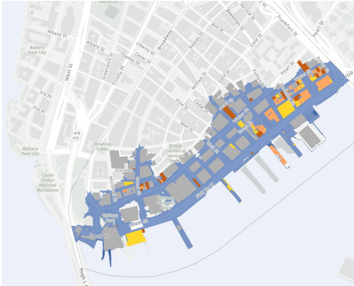
Figure 6: Repetitively Flooded Buildings
