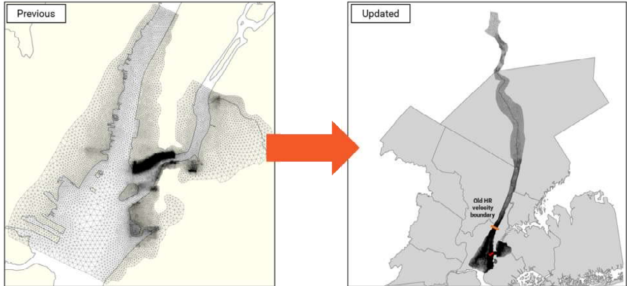
Figure 28 - Comparison plot of 2D D-Flow FM model mesh (left) to the 3D D-Flow FM model mesh (right) that shows the Hudson River extension to the northern boundary of the ADCIRC+SWAN model domain
