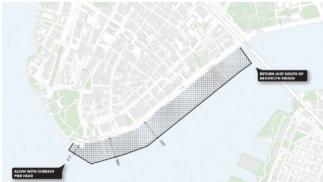
Figure 9 – Example 500-ft simple shoreline typology. This alignment was only intended to assess the potential hydrodynamic impacts and was not a project alignment under consideration at any point.
