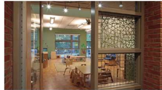
Green lights signal to children to open windows for passive ventilation.
