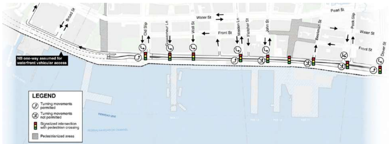
Figure 16. At-Grade Avenue/Boulevard Signals and Turn Lanes
