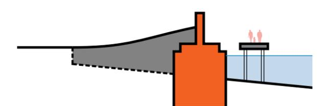
Raised Shoreline (New Bulkhead and Exposed Floodwall)
