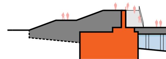
Raised Shoreline (Caissons and Buried Floodwall)
