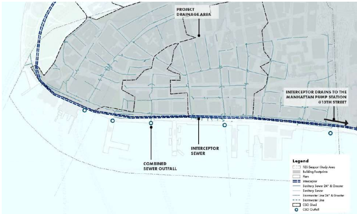
Figure 5. Existing Drainage Infrastructure in the Study Area
