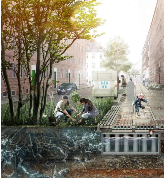
Climate Tile; Copenhagen, Denmark Stormwater Management + Neighborhood Improvements
